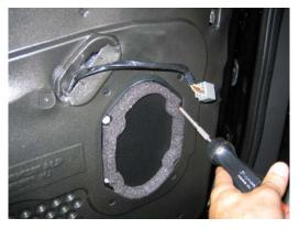
Remove speaker from door panel. Remove screws and unplug connector
